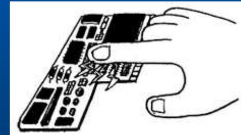
Electrostatic discharging from worker to PCB during production.
